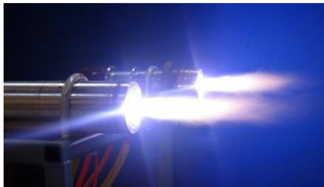
Figura 13 Antorcha de Plasma. Ref: Pyrogenesis Engine.
